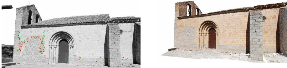
Fig. 11. Left: Back projection error on pixels with a magnification factor of 10. Right: Texture mapping as the result of the fusion of both sensors
