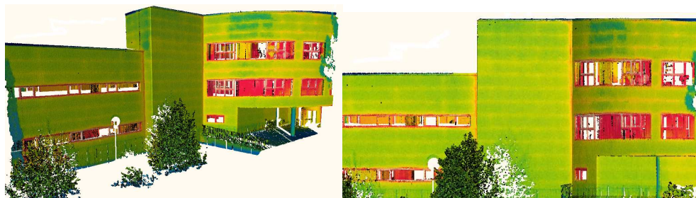
Fig. 19. Hybrid products from the fusion sensor: 3D thermal model (Left); thermal orthophoto (GSD 5 cm) (Right).
