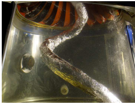
Fig. 2. Development of a cavitating helical vortex downstream the runner of a Francis turbine at partial load
