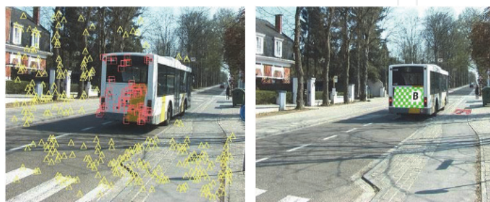
Figure 22. Augmented reality and 3D estimation through points relative movements in (Ozden, Schindler, & van Gool, 2007)
