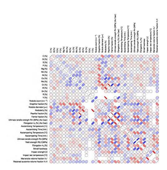
Fig. 12. The input and output correlation matrix. The blue color represents the positive correlation while the red color represents the negative one; the deformation size correlation, of the circle (ellipsoidality) and the color saturation indicate the correlation strength (Murdoch & Chow, 1996)
