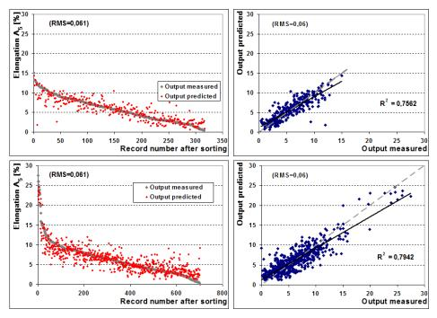
Fig. 15. The distribution of the real results and the predictions of the elongation variable for a) the data set without replacement; b) the data set after replacement
