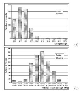
Fig. 13. The proportions of the numbers of records in the specified ranges of the output variables a) elongation [%], b) ultimate tensile strength [MPa] before and after replacing the missing and empty values
