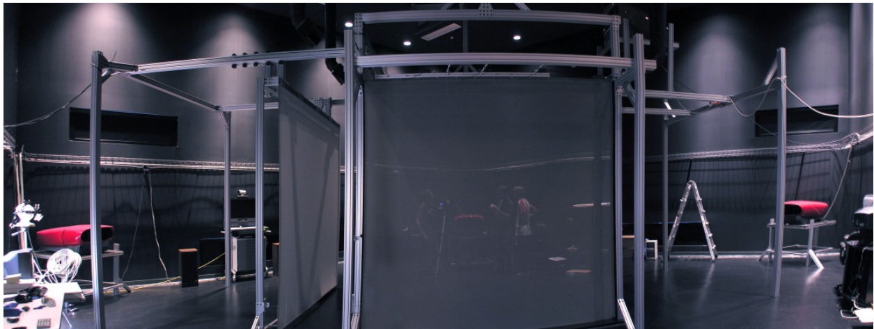
Figure 4. A room-size immersive system where the user stands up in a cube with stereoscopic images retro-projected on its wall to create a very strong sense of presence.
