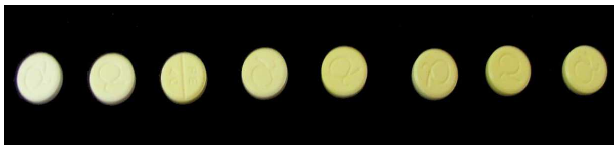
Fig. 4. Progression of colouration of frusemide tablets exposed to fluorescent lighting over an eight week period from left (week 1) to right (week 8)
