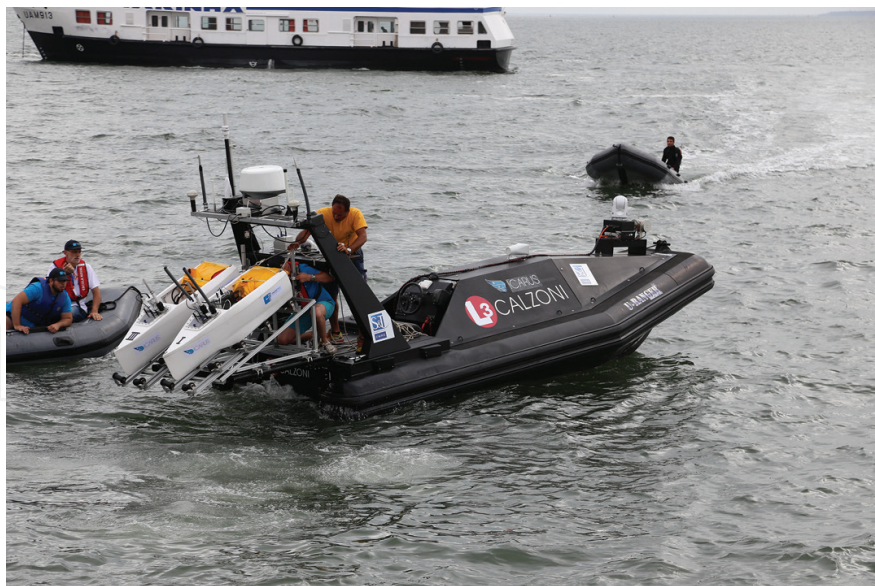
Figure 13. Two UCAPs mounted on the deployment system installed on the U-RANGER (source: ICARUS).
