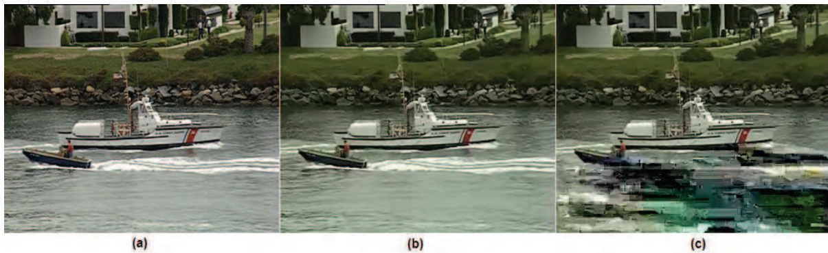
Fig. 15. Subjective quality: (a) Coastguard original frame number 2191, (b) VP7 encoded-decoded, (c) VP7 reconstruction with packet losses.
