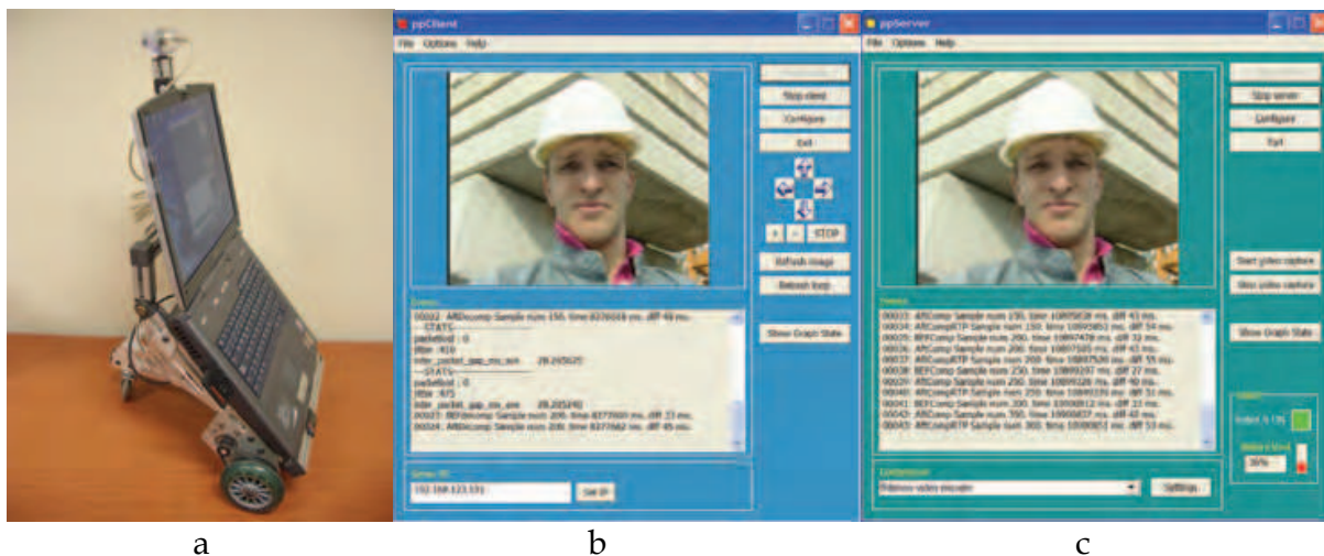
Fig. 2. (a) ER1 and laptop, (b) Client application, (c) Server application.
