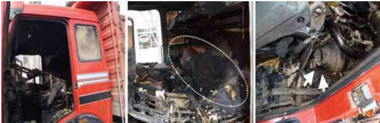
Fig. 25. A 48-year old male truck driver (ellipse) was found dead due to a fire in a truck parked in an open area of the truck garage. Scene investigation revealed that the cause of fire was broken supplementary heater (arrows) in the truck.
