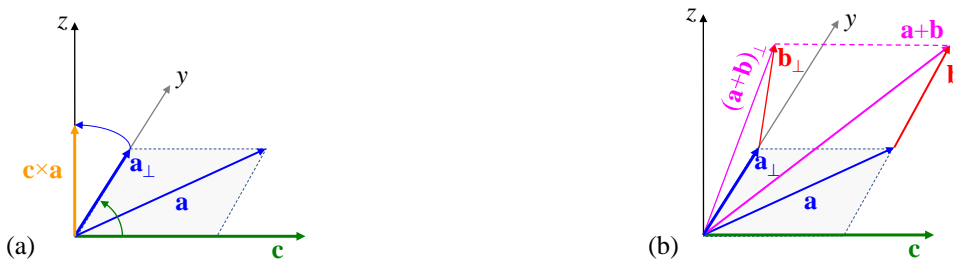
Figure 12.3 (a) Construction of a cross product. (b) The cross product of a sum: The projection of \mathbf{b} slides its tip to the y - z plane.
