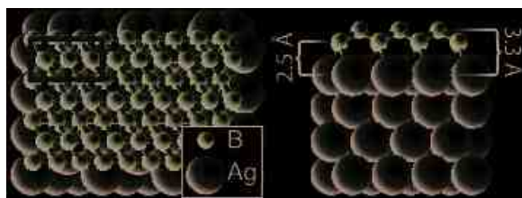
Figure 3. The borophene structure on a silver substrate: the top and side views of the monolayer structure (unit cell indicated by the box) [16].
