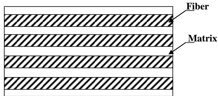
Fig. 1.1 Structure of a fibrous composite
