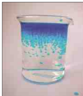
Figure 9.2 Laboratory experiment showing the formation of salt fingers. Assistance with the experiment provided by Christoph Funke.
