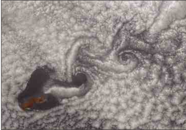
Figure 3.13 Vortex street in the lee of Guadalupe Island in the eastern Pacific. The vortices are formed by the same shear instability that causes a flag to flutter in the wind, the sinuous instability of a plane jet. (NASA)
