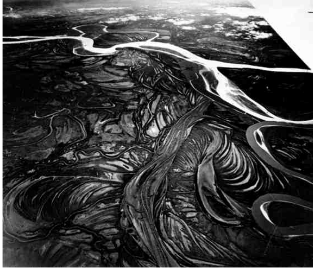
Figure B.1 Braided drainage pattern near the confluence of the Yukon River and Koyukuk River, Alaska. The Koyukuk River (dark) joins the silt-laden Yukon River (lighter) at the right (Image by U.S. Army Air Corps, 1941).
