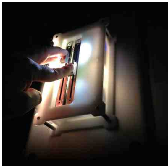
Fig. 9.2 FireFader is a force-feedback device with two motorized faders. It uses open-source hardware and is based on the Arduino platform, so it can easily be reconfigured for a wide variety of applications
