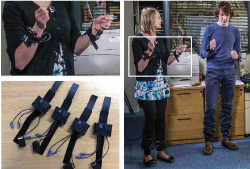
Fig. 11.2 A set of four Haptic Bracelets (lower left). Two users listening to music (right) and feeling what each limb of a drummer does and when—with the Haptic Bracelets acting as a Haptic iPod (upper right)
