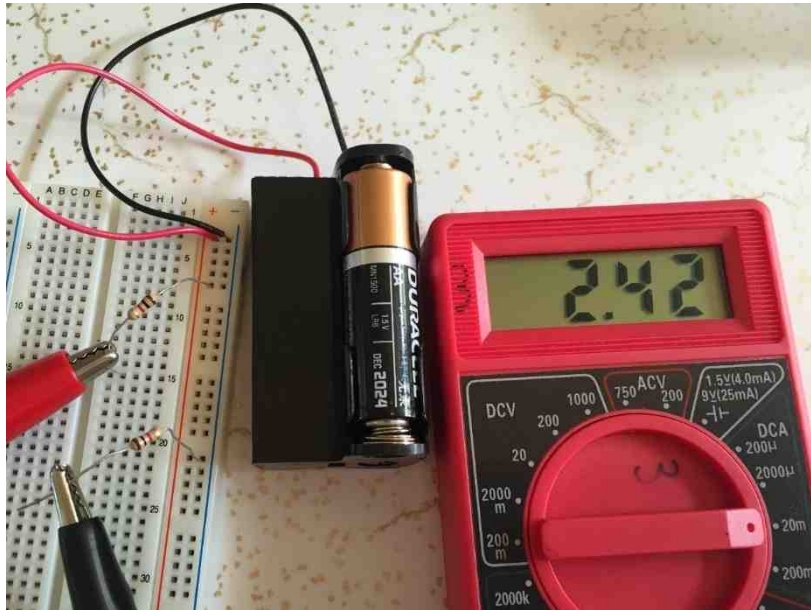
Figure 1.8: Circuit showing current measured with a Multimeter.
