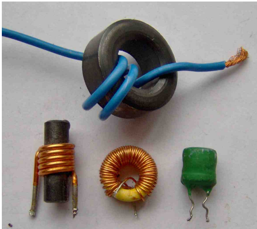
Figure 3.8: Inductor examples. Photo © FDominec and used under a CC BY-SA 3.0 license: https://commons.wikimedia.org/wiki/File:Electronic_component_inductors.jpg
