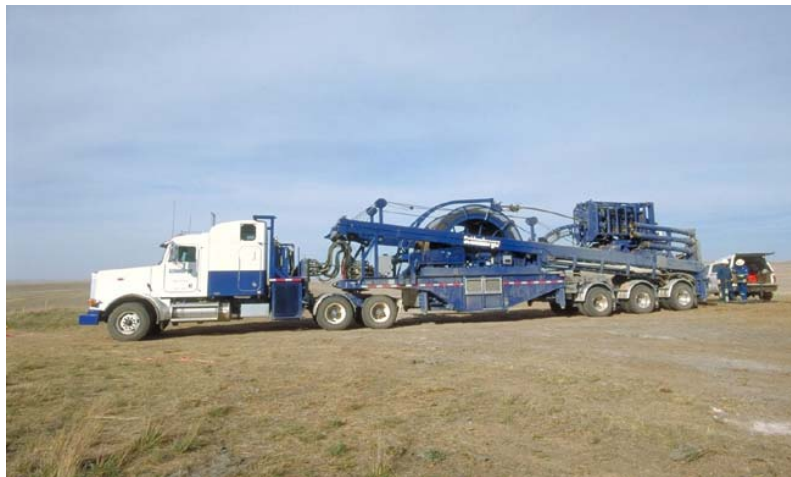
Fig. 2.3—A coiled tubing mast unit is rigged down. ‡
