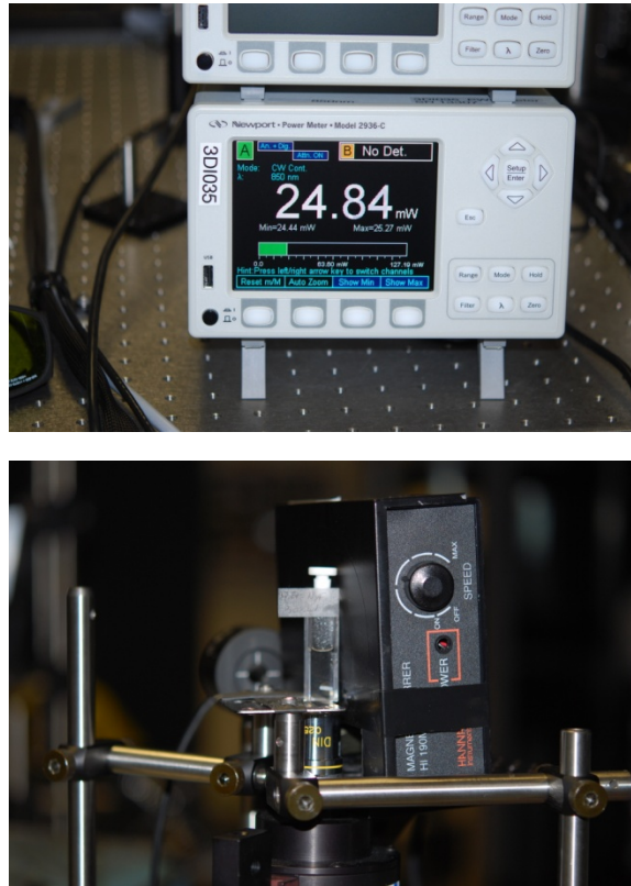
Figure 6.2.1.1. Scattering measurement for the sample 1%Er: NaYF 4 30 wt% dispersed in 1.468.
