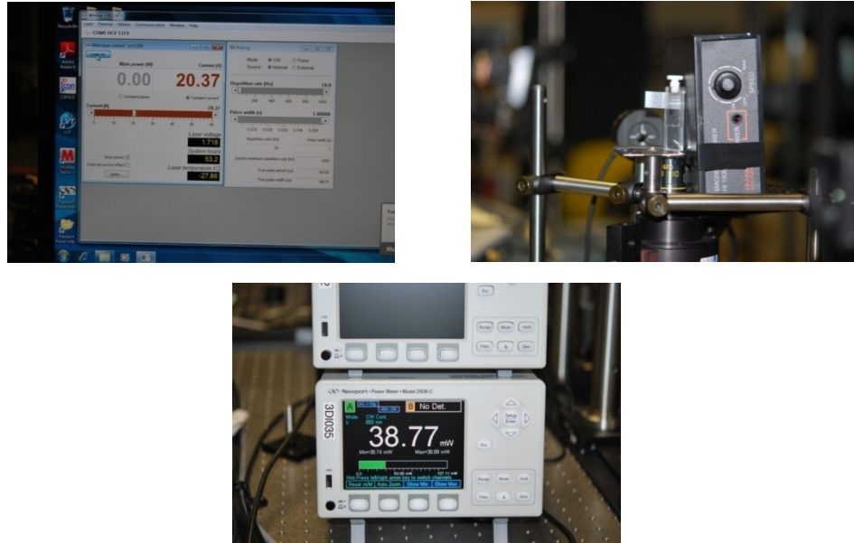
Figure 5.3.2.3. Measurement setup for the transmission test for the sample 0.5% Er: LLF10 wt% dispersed in 1.45.
