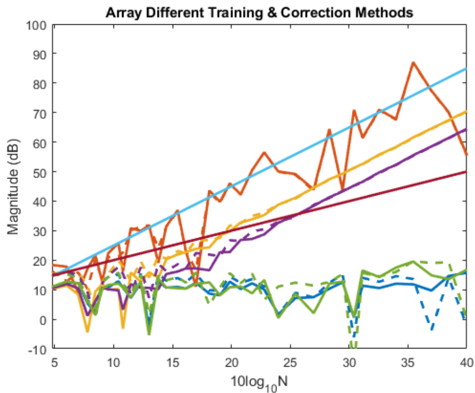
Figure 51: A performance comparison of the different proposed techniques for array-level decorrelation of odd-order spurs for arrays with Gaussian distributed elements, in this simulation the standard deviation was 0.1 and the results were averaged over ten simulations. The cyan and magenta lines are 20\log_{10}N and 10\log_{10}N , respectively. The remaining solid and dashed lines are the resulting magnitudes of the spurs after NLEQ was applied to the array for the methods of individual element correction (blue), single element coefficient correction (orange), average coefficient correction (yellow), root-average coefficient correction (purple), and hand-tuned root-average coefficient correction (green).
