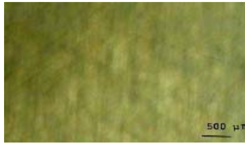
Fig. 5.10 Nomarski image of substrate surface after 17 min polishing with CMP-I.
