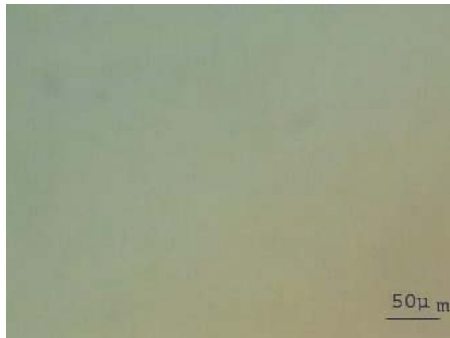
Fig. 5.11 Nomarski image of polished substrate surface after 25 minutes polishing with CMP-II.
