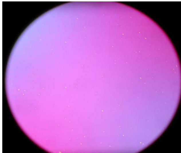
Fig. 2.8 Nomarski micrograph of an as-grown PbSe epilayer on Silicon substrate.
