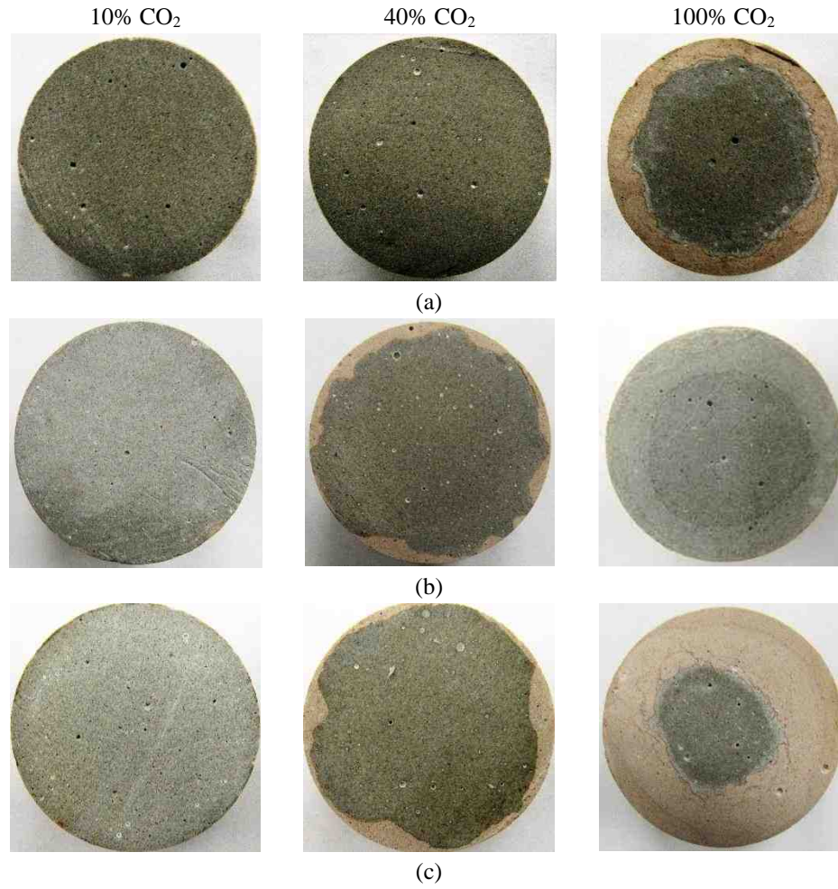
Figure 4.36 Visual degradation of Class G cement due to variation in CO 2 gas composition at 350°F and: (a) 3000 psi; (b) 6000 psi; (c) 9000 psi
