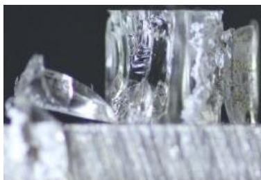
Figure 65. Typical failure PDMS sample under compression.
