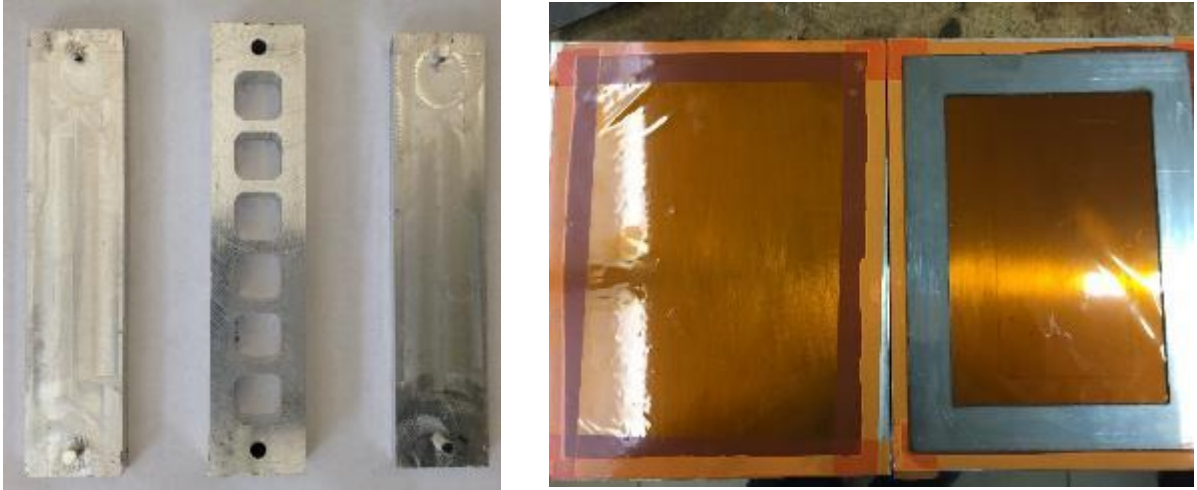
Figure 7. (a) Compression sample mold (b) Tension sheet mold.
