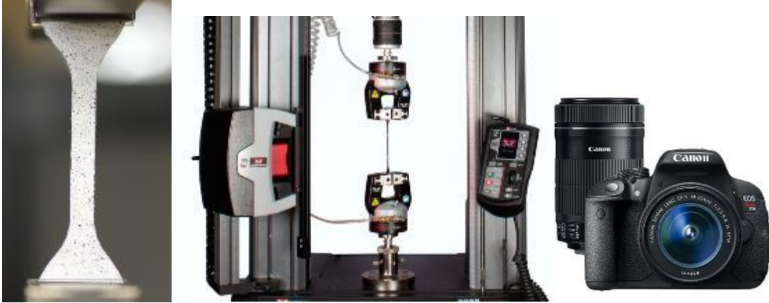
Figure 17. (a) PDMS sample setup in tension (b) Instron Single Column Machine (c) Canon® EOS Rebel T5 Camera[38].
