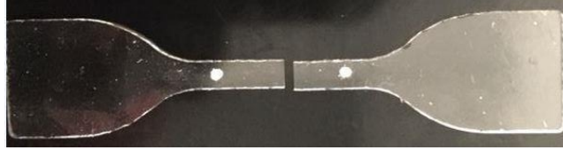
Figure 62. Typical failure PDMS sample under tension.
