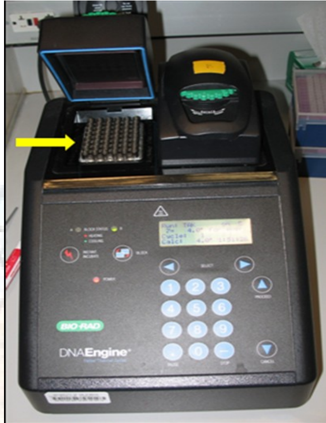
Figure: Image of a PCR thermocycler (BioRad Company). The yellow arrow indicates the block where PCR tubes are inserted.
