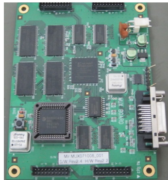
Figure 5.10: The mux board used is custom built by the Army Research Lab. It is used to select whether to use the custom flight controller on the Odroid or the Pixhawk flight controller for vehicle actuation.
