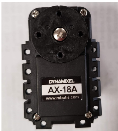
Figure 5.8: The AX-18A Dynamixel servos mounted on the tilt-rotor.
