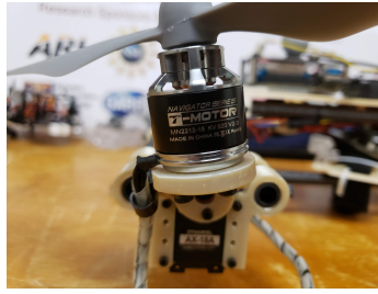
Figure 5.5: Tiger-Motor MN2212 920KV motors.
