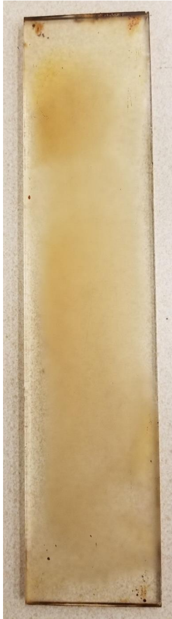
Figure 4.17: Appearance of window glass of 50J50C fuel
