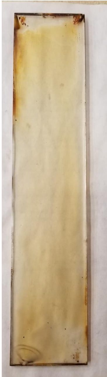
Figure 4.18: Appearance of window glass of 25J75C fuel
