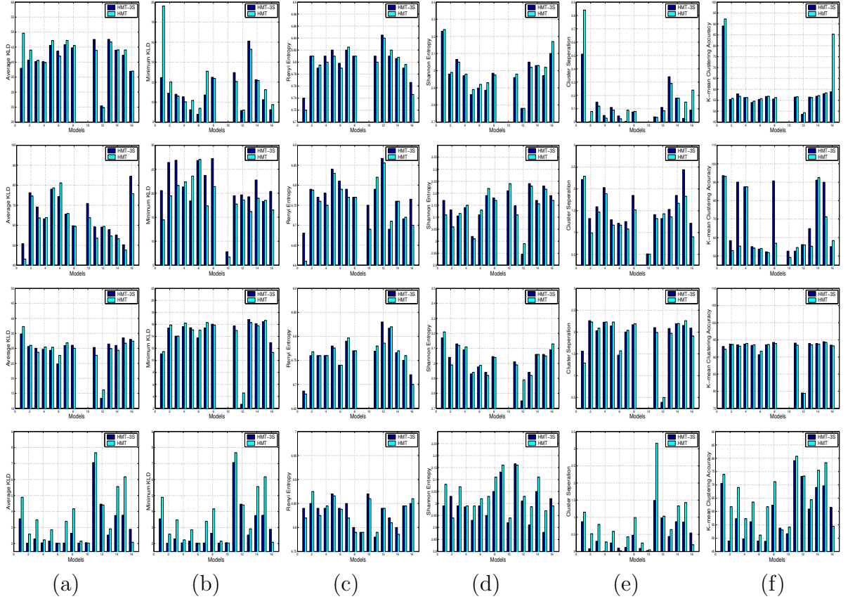
Figure 4.5: Cluster divergence in different model specifications and spaces, where model indices from 1 to 16 are corresponding to: mosaic image (Mosaics 5 to 8 from top to bottom), D9, D12, D15, D16, D19, D24, D29, D38, D68, D84, D92, D94, D112, Sand, and Mix. (a) Average KLD. (b) Minimum KLD. (c) Renyi entropy. (d) Shannon entropy. (e) Cluster separation. (f) K-mean clustering accuracy.
