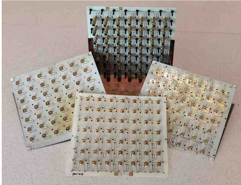
Figure 4.14: Depiction of three boards and how they are mounted on the antenna array.
