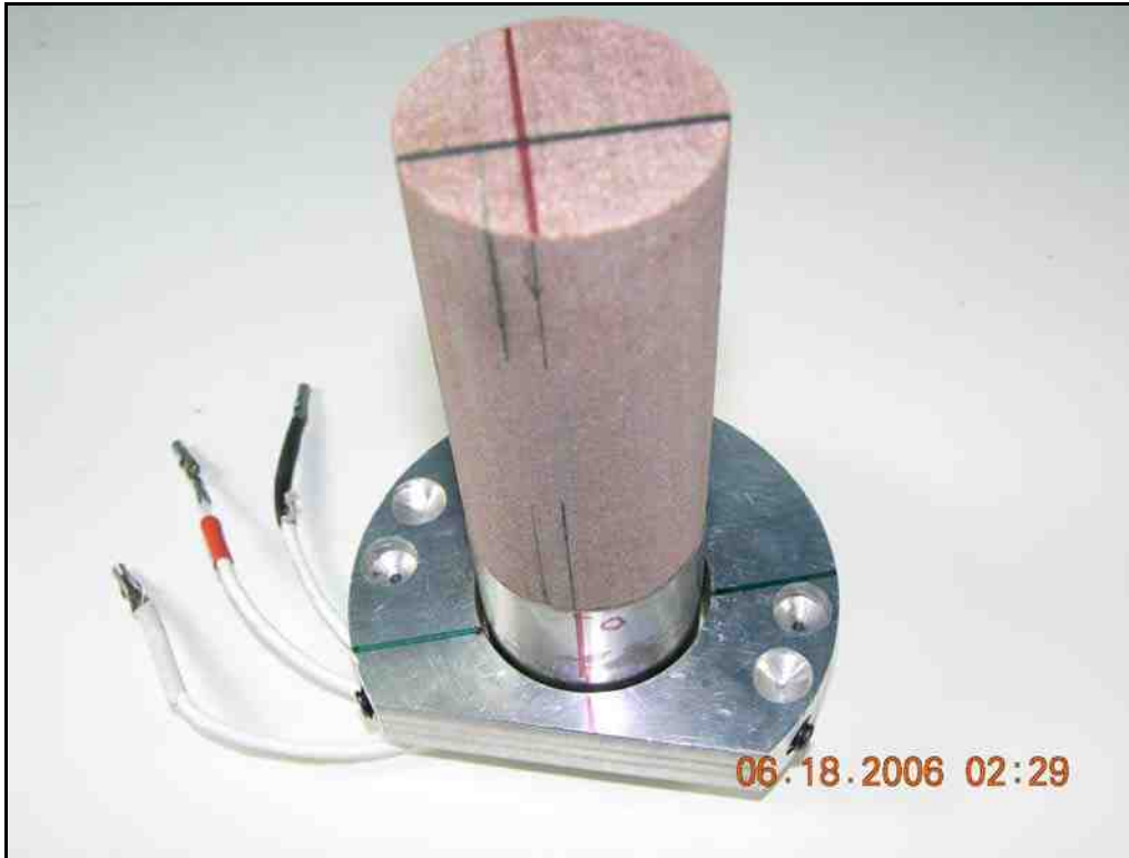
Figure 3-8: Alignment of sample bedding with the polarization of the shear crystals (horizontal sample).
