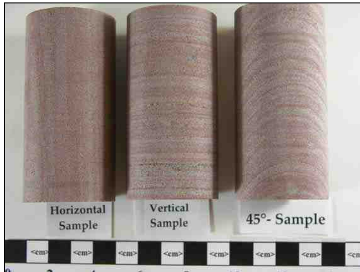
Figure 3-2: Pictorial view of the candidate samples submitted for testing with designated directions. Notice the finely-layered dipping beds reflecting the assumption of their inherent apparent anisotropy.
