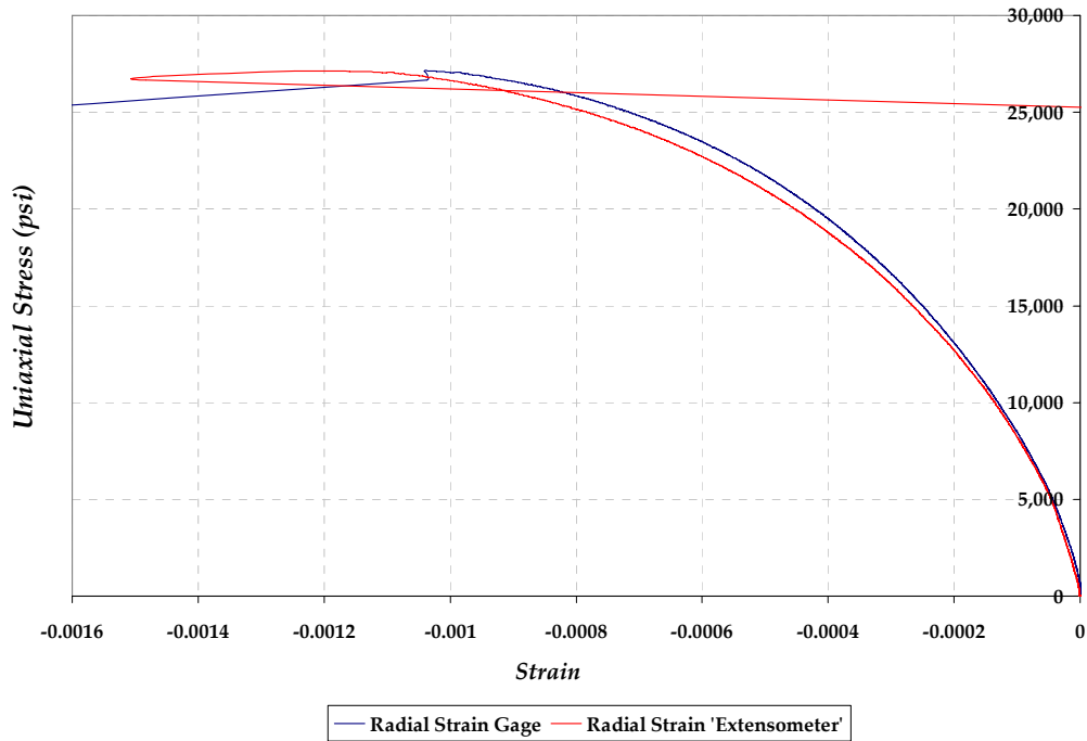
Figure 3-21: Comparisons of the circumferential strain measurements from strain gages and extensometer, horizontal sample H-2.
