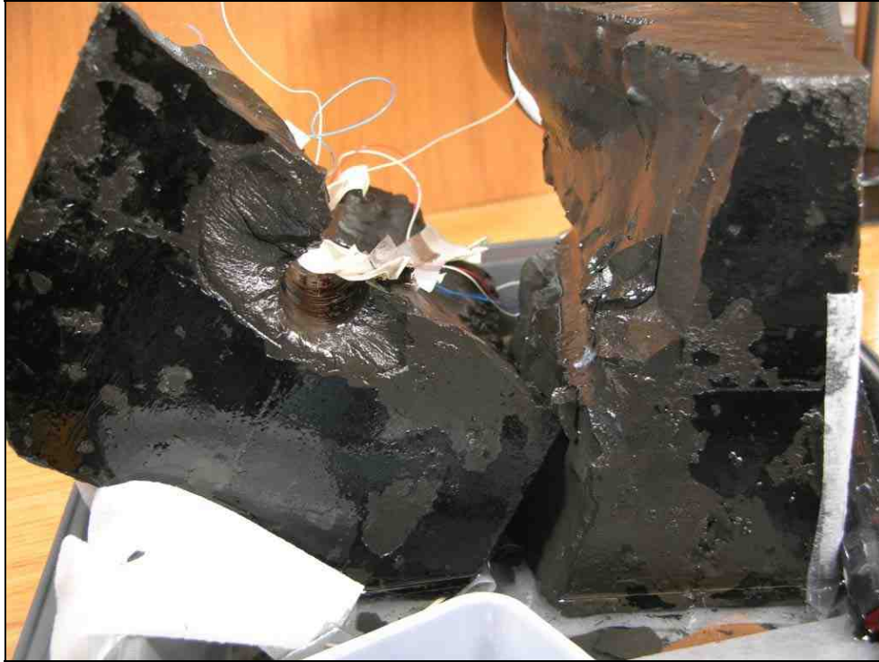
Figure 6-58: Failure of the Pierre shale block during preparation and instrumentation (the orientation of the bedding is 60^\circ relative to the borehole axis).
