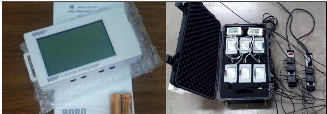
Figure 2-10: Utilized DAQ for recording airflow measurements.
