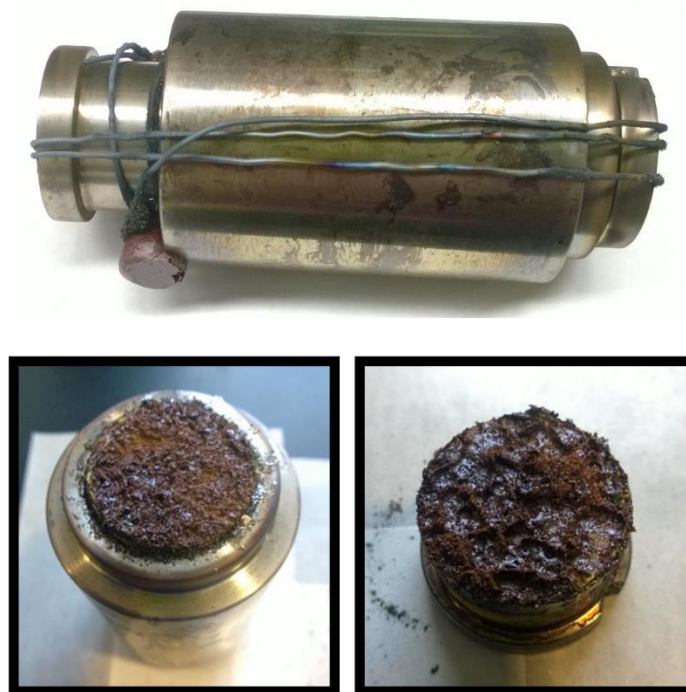
Figure 5.2.9: S-PCP-50 heated at 300\text{ }^{\circ}\text{C} furnace for five hours. Top: die immediately after removal from furnace. Bottom: foamed material remaining inside the die.
