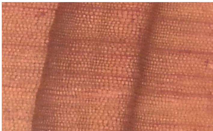
Figure 2: Image of annual ring (left) and false ring (right)
