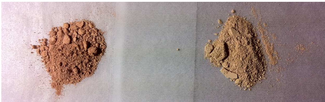
Figure 15 (above). Unreacted iron fumarate (left) and iron fumarate that has been reacted with an excess of phosphate (shown on right).
