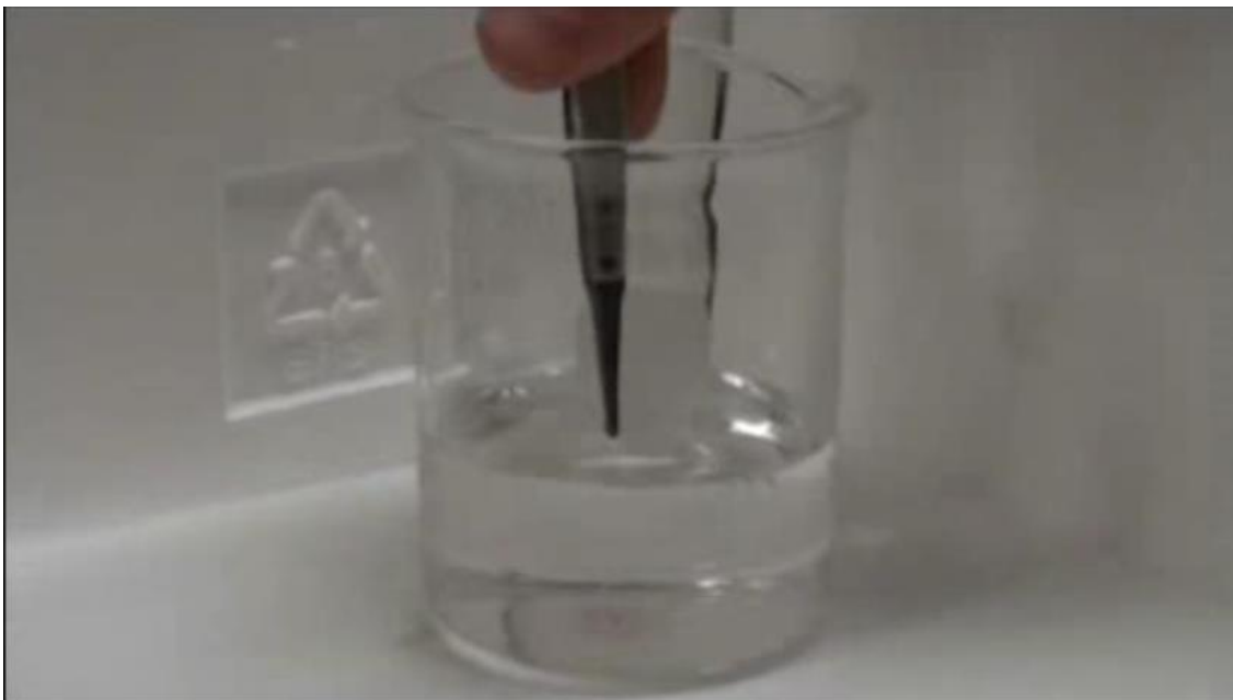
Figure 3.6 Unused HRP loaded thin film being placed in guaiacol assay solution.
