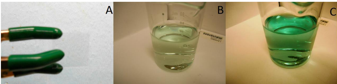
Figure 3.10 A) Pristine silica sol-gel thin film coating glass coverslip loaded with cytochrome C; B) ABTS assay solution 5 minutes after a cytochrome C loaded thin film was introduced; C) ABTS assay solution upon the consumption of all ABTS as \text{H}_2\text{O}_2 is in excess in the ABTS assay solution. Figure adapted from ref. 22.
