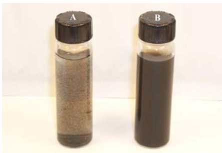
Figure 3-1. Suspensions of unmodified pristine single-walled carbon nanotubes ( A ) and polymer-modified single-walled carbon nanotubes ( B ).
