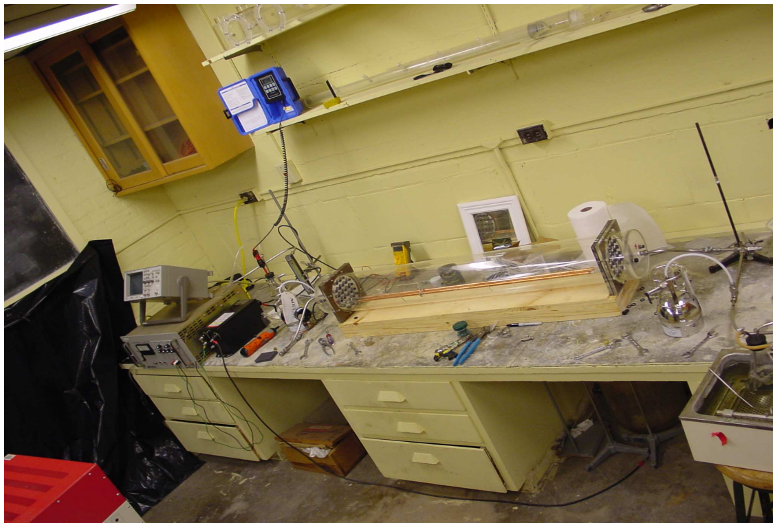
Figure 3-2: Experimental set-up, from left to right; AC power supply, Transformer, Plasma reactor
