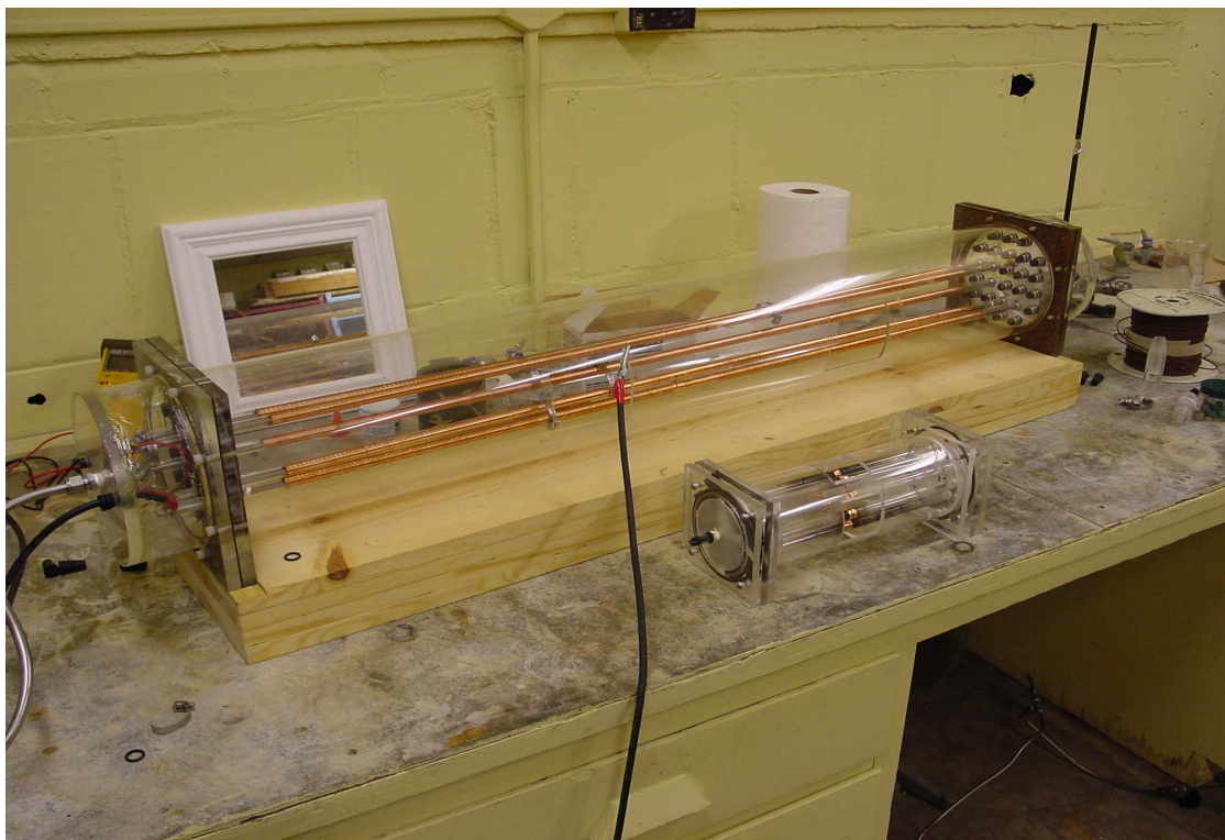
Figure 3-9: Quartz casing with two reactor tubes inside it
