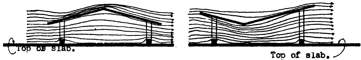
Double Roof - Air Flow Pattern
