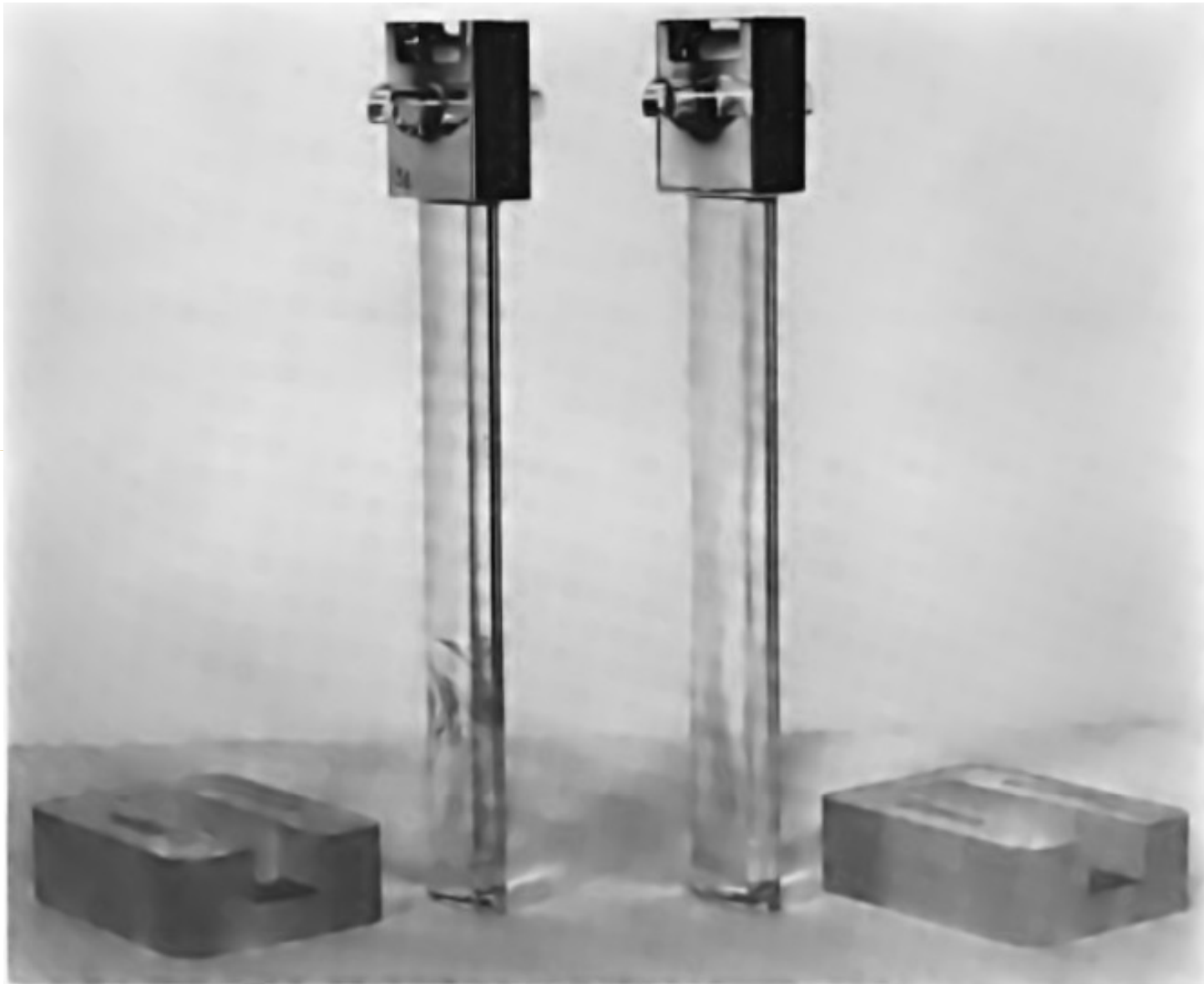
Quartz pendulums used in the Gulf gravimeter, 1929. Accurate to better than one part in 10 million.
