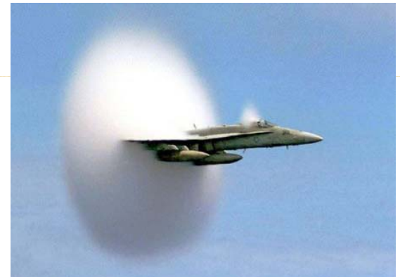
Water condensing in a shock wave
