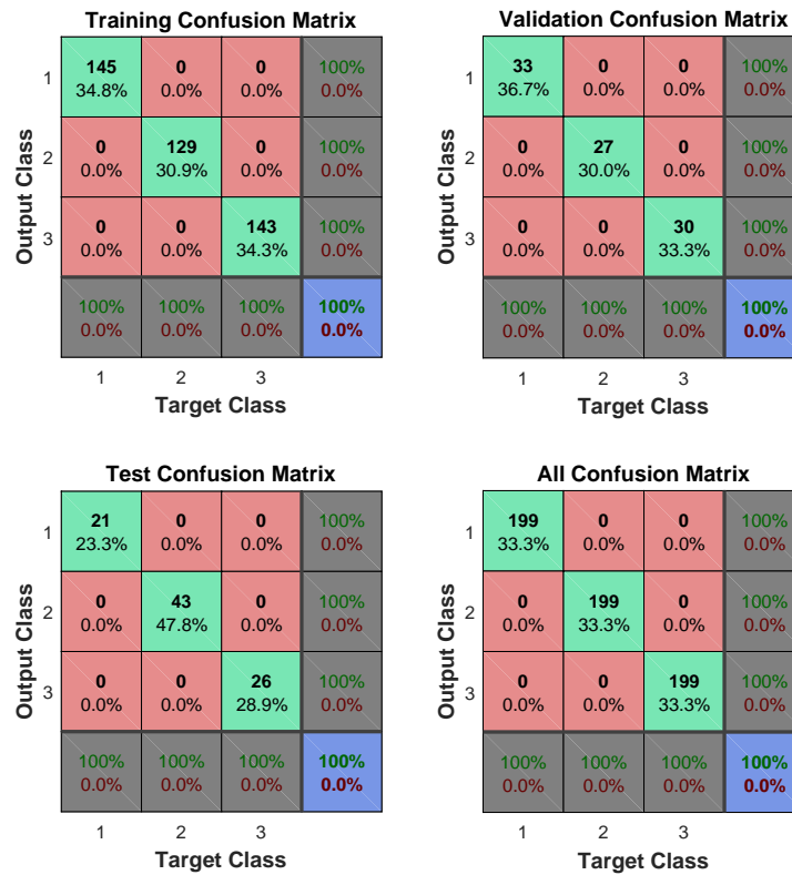
Figure 5.20: Load Fault Classification Network Confusion Matrix
