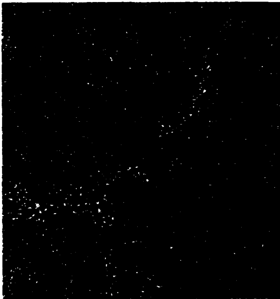
Figure 2.16 Unreacted polished (5 \mu\text{m} ) Carrara marble showing an overall uniform surface. [150 \mu\text{m} X 150 \mu\text{m} ]
