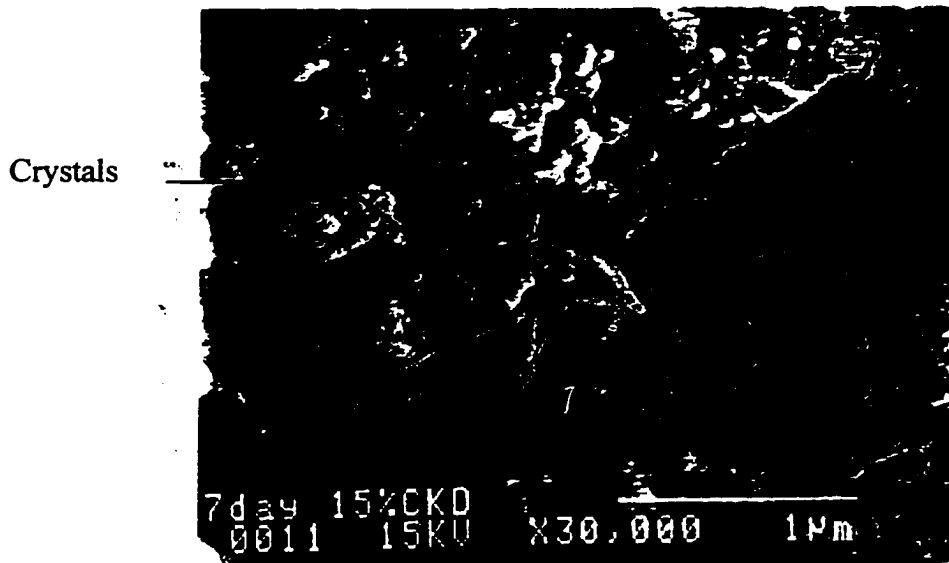
Figure 5-25 Micrograph of the 7-day Cured Aggregate Stabilized with 15% CKD
