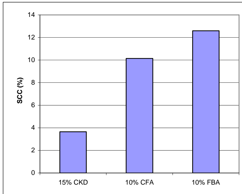
Figure 5-17 Effect of different stabilizing agents on SCC
