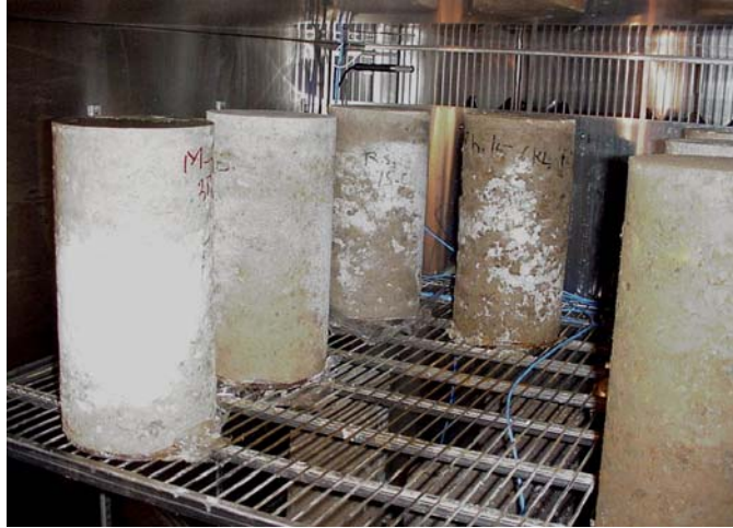
Figure 3-1 Specimens subjected to freeze-thaw cycles using a rapid F-T cabinet
