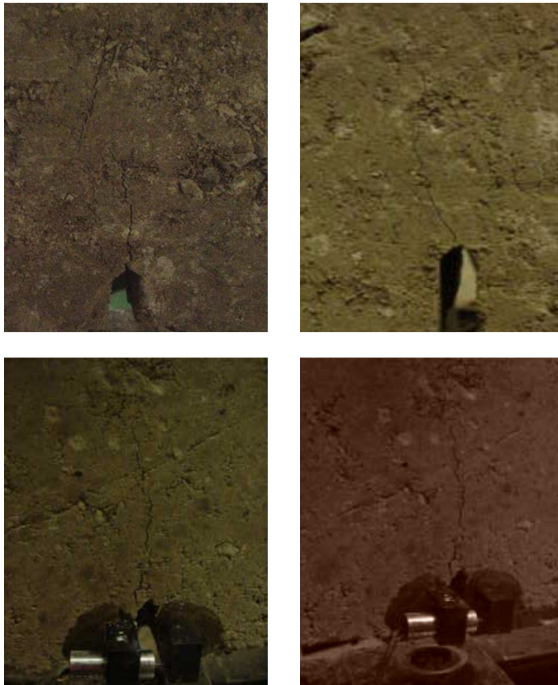
Figure 6-8 Cracks path during the fracture energy test
