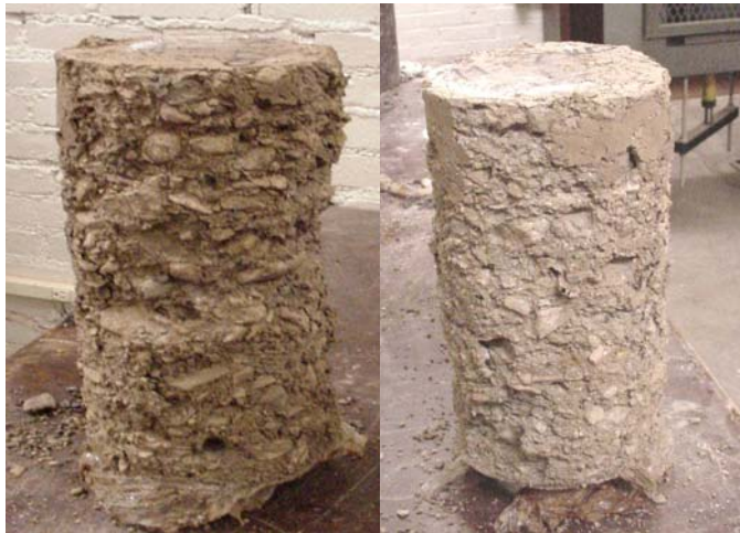
Figure 3-2 Meridian aggregate specimens stabilized with 15% CKD and subjected to 30 F-T cycles; specimens could not be tested due to excessive degradation
