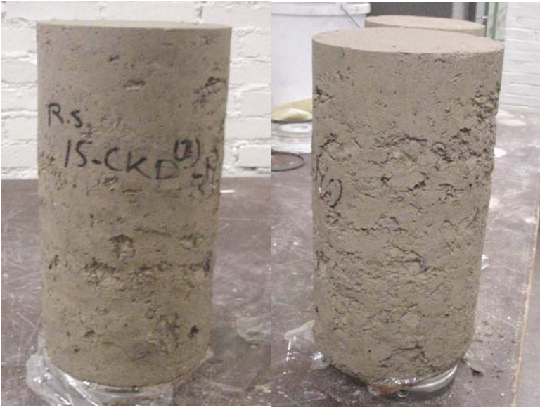
Figure 3-4 Richard Spur aggregate specimens stabilized with 15% CKD and subjected to 30 F-T cycles
