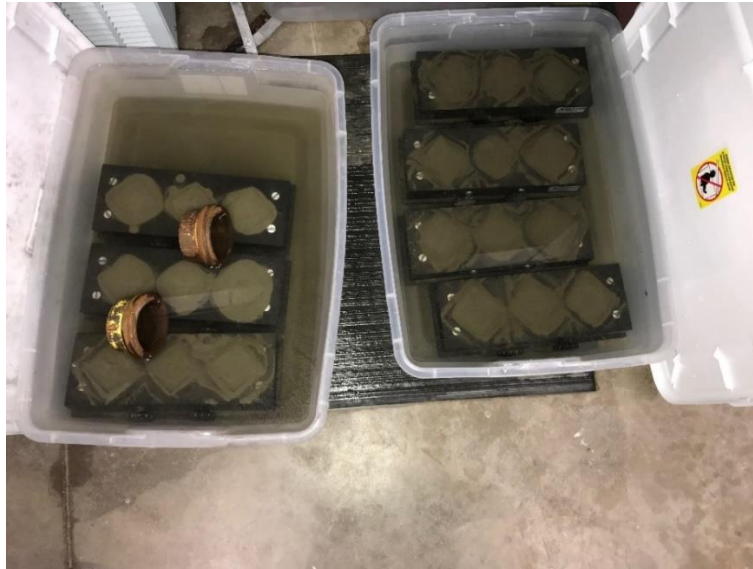
Figure 80: Prepared samples for Unconfined Compressive Strength and Ultrasonic Cement Testing.
