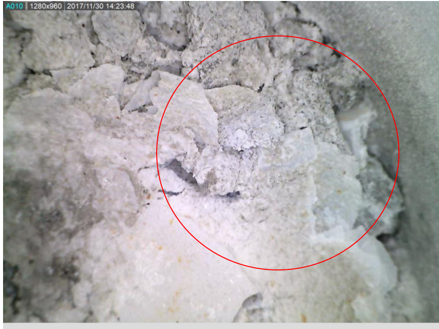
Figure 63: Fly ash cement showing leak position (Small Setup 1 Experiment 6).
