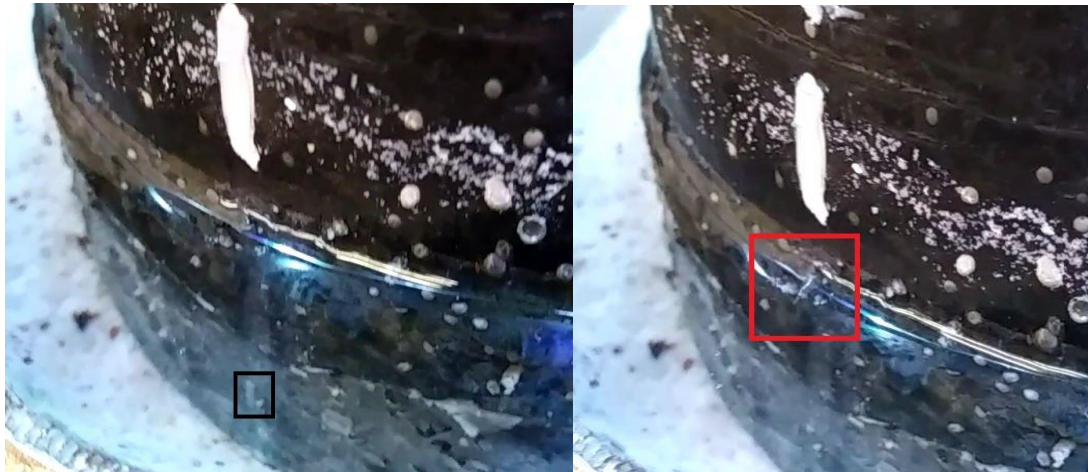
Figure 49: Left - Gas bubble travelling from cement sheath through water to surface. Right – Travelled gas bubble bursting at surface.
