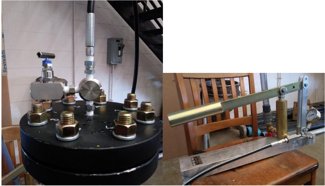
Figure 48: Setup for ballooning inner pipe. Left – Connection from hand pump to inner pipe. Right – Hand pump used to pressure the inner pipe of Setup 1.
