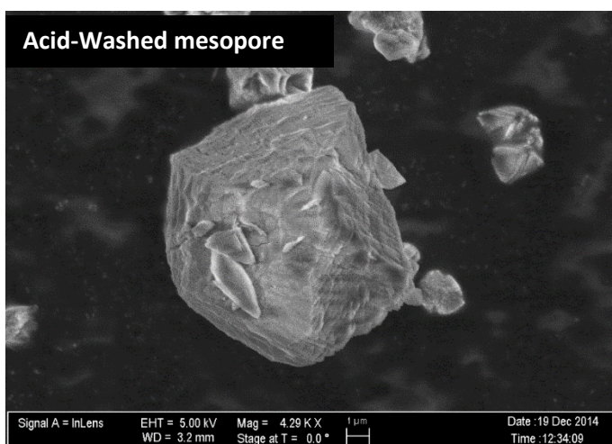
Figure 28 : SEM image of the acid washed mesopore sample
