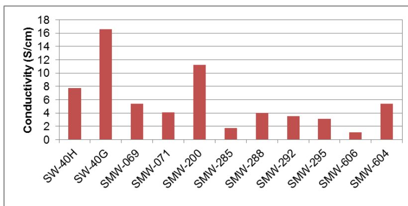
Figure 3.4. 4-Point Powder Probe Conductivity of pure CNTs as received.
