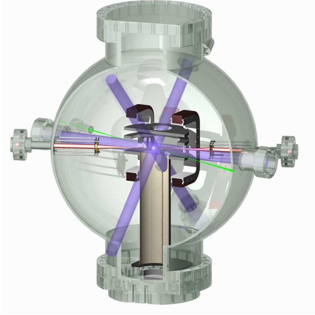
Figure 3.10: To scale rendering of the spectrometer located in the vacuum chamber. The spectrometer is sectioned for viewing. The bright spot in the center represents the MOT. The spectrometer is formed around the MOT with the flight tube extending downward towards the MCP detector. The anti-Helmholz coils are also depicted. The lens systems are used to focus a CO 2 laser to form an optical dipole trap.
