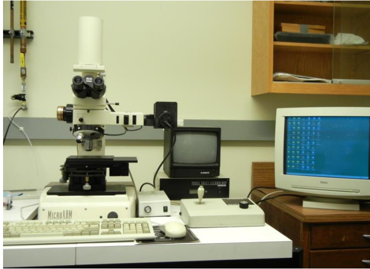
Figure 3-6: MicroXAM, optical laser interference microscope [25]
