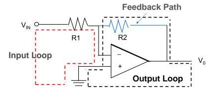
$$V_0 = -\frac{R_2}{R_1}V_{IN}$$
