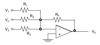
$$V_0 = -\frac{R_F}{R_1}V_1 - \frac{R_F}{R_2}V_2 - \frac{R_F}{R_3}V_3$$
