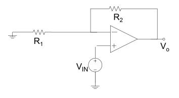
$$V_0 = \left(1 + \frac{R_2}{R_1}\right) V_{1N}$$
