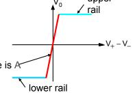
Can add negative feedback to perform an "operation" on input voltages (addition, integration, etc.): **operational amplifier**
