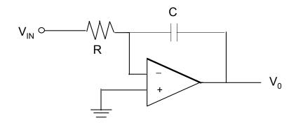
$$V_{O}(t) = -\frac{1}{RC} \int_{0}^{t} V_{IN}(T) dT + V_{C}(0)$$
