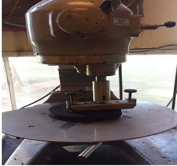
FIGURE 9 Raveling Test Setup
