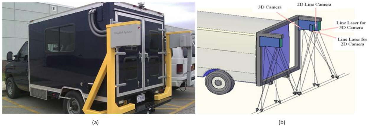
Figure 4.1 Photographs of (a) DHDV exterior appearance; (b) Pavevision3D working principle.
