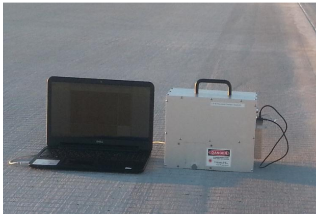
Figure 3.6 LS-40 Surface Texture Analyzer in operation
