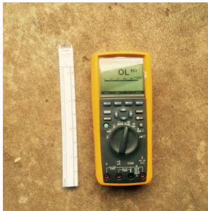
Figure 3.5 eTape liquid level sensor and FLUKE 289 true RMS multi-meter
