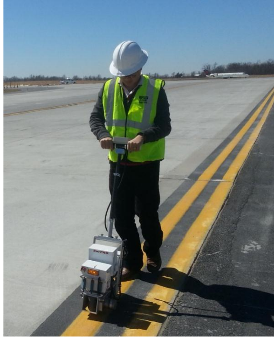
Figure 3.7 SurPro3500 walking profiler in operation
