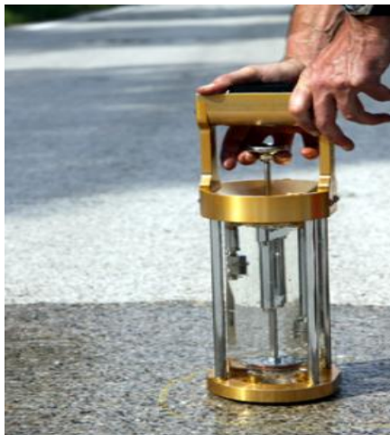
Figure 2.5 Outflow Meter (ASTM E 2380)
