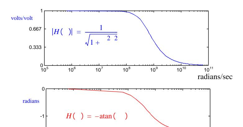
• The steady state response of a cosine input signal is modified in terms of phase and magnitude as displayed on the plots
