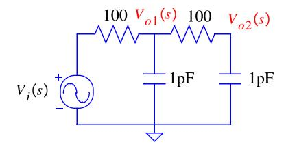
$$H_1(s) = \frac{\frac{(1+10^{-10}s)}{10^{-20}}}{s^2 + s(0.03 \times 10^{12}) + 10^{20}} = 10^{20} \frac{1 + \frac{s}{10^{10}}}{s^2 + s(0.03 \times 10^{12}) + 10^{20}}$$
